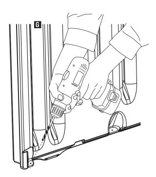
Align the lap joint between Repeat Left Side (C) and Front Left Side (G).
